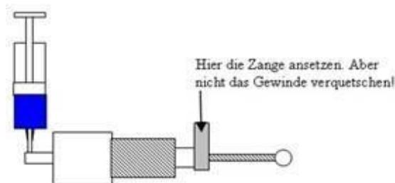
Now the hose is placed under the headlight under liquid on the connection of the cylinder. Push firmly until it stops and remove the locking pliers, done! The system pressure is then built up by the spring tension of the cylinder. The pressure could not have been greater when the system was manufactured, otherwise the push rod would have stuck out of the cylinder permanently. The whole thing is done again for the other side.
