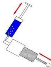
When you let go of the plunger of the syringe, the spring in the cylinder pushes the rod and thus the plunger and the liquid back into the syringe. If there is air in the cylinder, it rises from the connection piece into the syringe and collects there. If you repeat this process a few times, the slave cylinder is empty.
