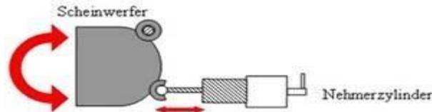
Use the knife to cut the two hoses on the master cylinder (switch in the interior) as close as possible (approx. 7 - 8 mm) before the connection. If possible at right angles to the hose core. Then the hose seals better later. The same applies to the slave cylinder.
